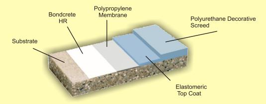
Bondcrete HR, Polysiloxane base coating all nanoparticles penetrate into cracks at the same time multiceramic technology base particles float on the top to bottom of the coating which creates water resistance and hydrophobicity.
