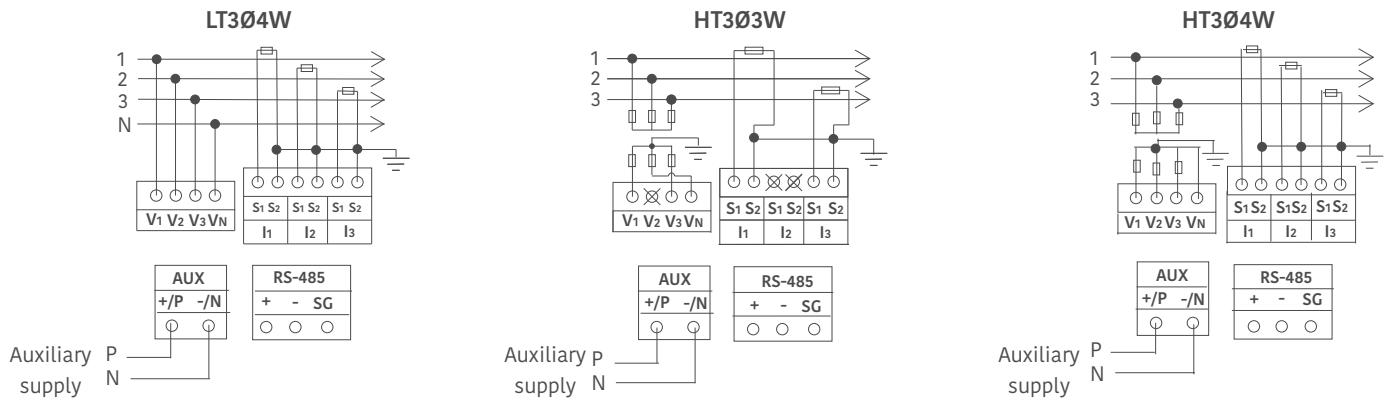
In case of CT/PT operated meter, ensure that meter is connected on secondary side of instrument transformer.
