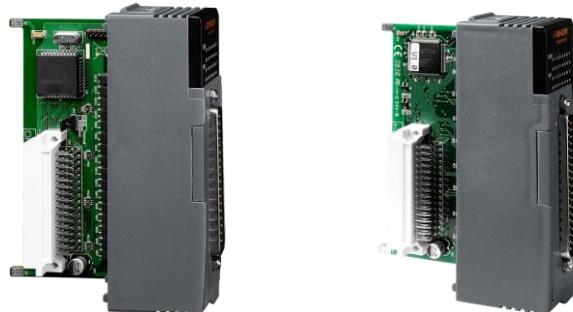
With different form factor, I/O modules can be classified to high profile and low profile. Basically, high profile and low profile modules that with same item number also have same I/O channel number.
