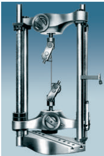
ATTACHMENT FOR TENSION TEST FOR WIRE ROPES.
