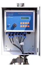
This Met Station is specially designed for Road weather monitoring applications. This system employs low power data logger system and rugged sensors for extreme road conditions. The system uses 12V operating voltage with a SLA battery backup while energy is harvested from a 12V/40W solar panel. Ethernet Interface is provided for Real time sensor monitoring. A stainless steel tripod stand is offered along with this system for robust mounting of data logger enclosure and sensors.
