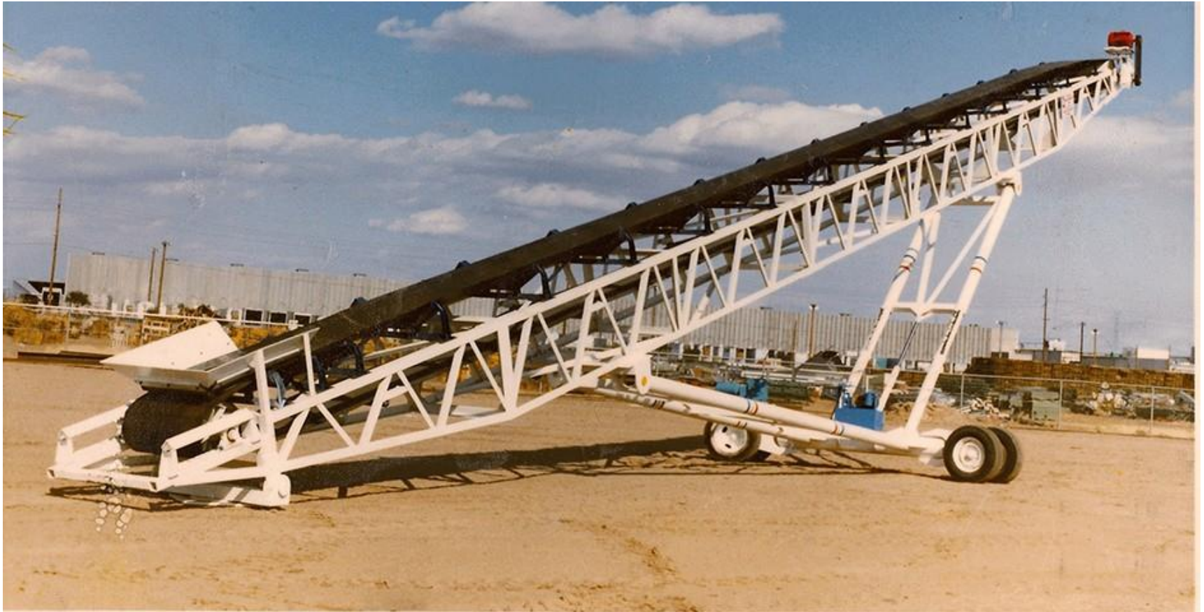
Portable Conveyors with Belt scale for Loading Applications at Port mines etc
