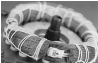
Fig. 28 Thermal switch incorporated in winding
