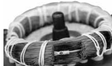
Fig. 26 PTC sensor incorporated in winding
