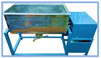
This blender consists of U shaped open drum with a rotating Shaft having Spiral ribbons/Paddle shaped Blades that rotates on a horizontal axis, mounted on a sturdy structure.
