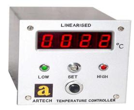
The Artech LIN 201 is a compact, sturdy and accurate instrument for temperature measurement and control, incorporating state of the art design techniques. A precision L.S.I.convertor chip digitizes the input signal which is then processed with reference to computer generated look up tables stored in a high density EPROM. Sensor break protection and cold junction compensation are standard features.
