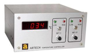
The Artech two set point Controller Model 231M is a compact, sturdy instrument useful for ovens, processing industries and laboratories. Sensor break protection and ambient furnaces, compensation are standard features. Set points are adjusted by means of two multiturn Potentiometers. Depressing each `SET' switch displays its relevant set point. In normal operation the display indicates actual temperature.
