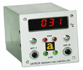
The Artech two set point Controller Model 201M is a compact, sturdy instrument useful for furnaces, ovens, processing industries and laboratories. Sensor break protection and ambient compensation are standard features. Set points are adjusted by means of two multiturn Potentiometers. Depressing each `Set' switch displays its relevant set point. In normal operation the display indicates actual temperature.
