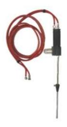
The ARTECH FEM-01 Fuel Efficiency Monitor is designed to monitor performance of boilers, heaters, furnaces, etc. It measures Oxygen, Carbon Monoxide and Temperature of flue gas. From these values it computes Combustion Efficiency, Excess Air and Carbon Dioxide values. It is suitable for all gas, oil & solid fuels.
