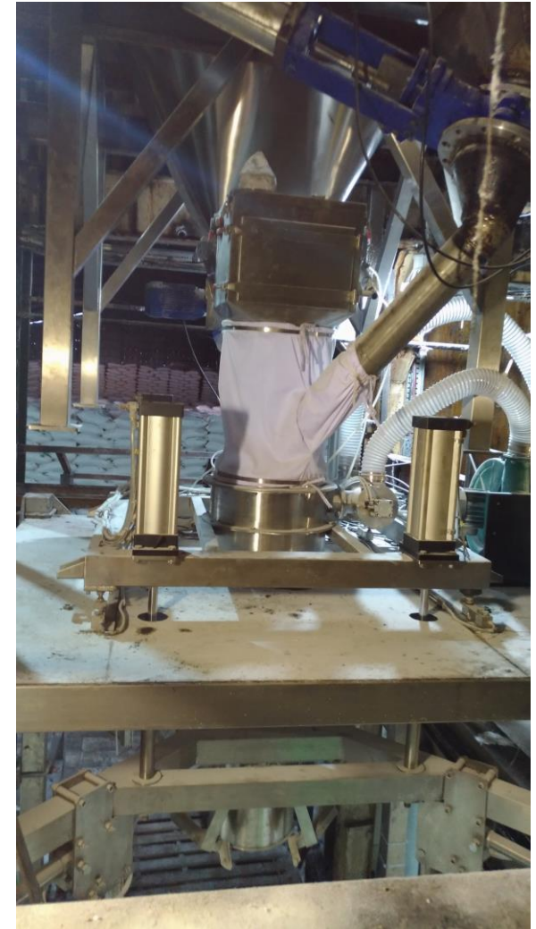
1t Jumbo Bag Bagging machine with Vibrating, Air Blowing, and Dust Collector units, installed at PT Dus Indonesia
