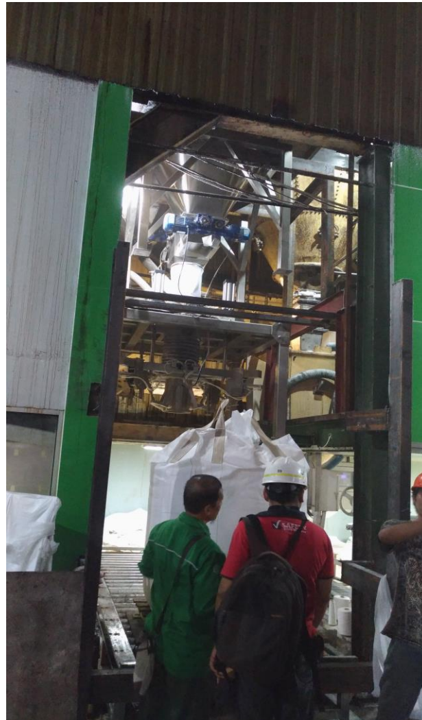
1t Jumbo Bag Bagging machine with Vibrating, Air Blowing, and Dust Collector units, installed at PT Dus Indonesia
