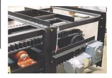
Weigh Feeders are widely used to feed bulk material in conveying system, in coal, metallurgy, cement steel & chemical Industry.
