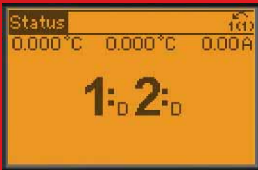
Read the compressor status directly from the display. D = Variable speed control, O = Off, R = Mains operation, X = Deactivated
