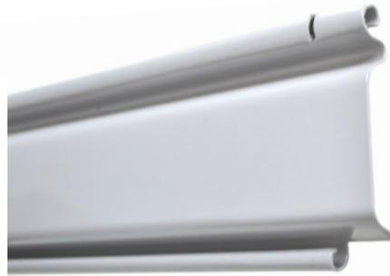
Single skin heavy duty Galvanized Steel slats (0.8mm, 1.00mm & 1.2mm thickness and 75mm) are interlocked and can be provided with optional wind locks. Where ventilation is required, perforations can be punched into the slats with holes of dia 3mm or 5mm to suit the application.
