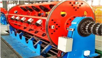
Automatic PLC Controlled Stranding Machines for Conductor making
