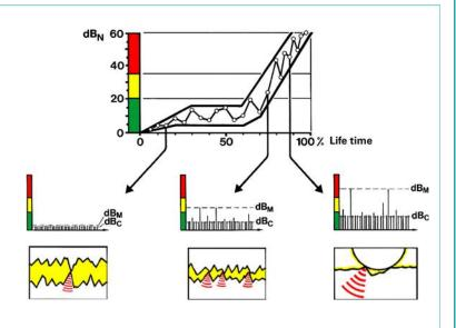
As defects in the bearing develop, the amplitude of shock pulses increases. Value exceeding the dBi characterizes the damage and is used to assess the condition of the bearing:
