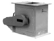
The equipment comes complete with a chute type feed hopper, adjustable feed regulation gate, magnetic drum and geared motor drive in a ready for use condition. Inlet and outlet openings are flanged for ease of connection to customers duct work. Double or triple totally enclosed machines can also be supplied if required by clients.
