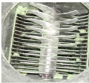
The Design of shape, material of construction, spacing / gap, Sizes, capacity, power all depends upon the type of material to be crushed.
