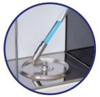
Laboratory holders provide dosing option of a sample, which is often of high value, directly into a vessel.
