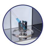
Holders have been designed to facilitate dosing samples directly into typical vessels such as: measuring flasks, round flasks, test tubes, titration vessels.
