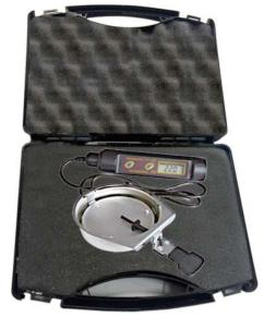
The main parameter determining the result of humidity content in a tested sample is the drying temperature. Placing the control thermometer directly above the drying pan enables reading the temperature close to the one of the tested sample. Thus, the adjustment is carried out in actual thermal conditions occurring on a typical analysis. A moisture analyzer adjusted using the control thermometer CTK 01 series operates precisely and with the highest accuracy.
