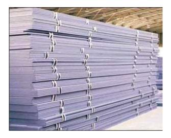
ABREX 400 is through solidified abrasion resistant steel with a regular hardness of 415 BHN. ABREX 400 steels are the most generally utilized of the wear safe evaluations. ABREX 400 shows a fantastic consolidation of high resistance to effect, workability, weld capacity and resistance to abrasion. ABREX 400 has around 3 times the abrasion resistance of normal steel plate and helps drawing out the administration life of mechanical parts.
