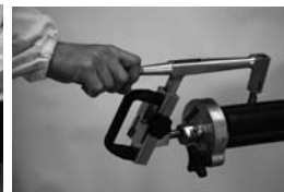
Phase 3 or mechanical scraping
