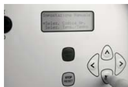
Phase 6 or setting up of parameters of manual welding
