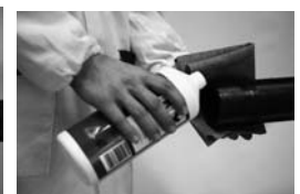
Phase 4 cleaning of the elements to be welded
