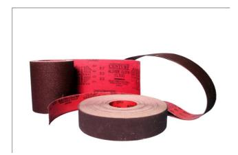
Made with Aluminium Oxide grains coated on X wt Light Drill Cloth with flexible bonding of synthetic resin. Grits available 24, 36, 50, 60, 80, 100, 120, 150, 180, 220, 320, 400, 600. Can be converted into belt, roll, Cloth Disc, Sheet, PSA Disc. Maximum Jumbo roll width 1410mm. Backing colour red.
