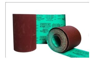
Made with Aluminium Oxide grains coated on flexible X wt Light Drill Cloth with flexible bonding of synthetic resin. Grits available 24, 36, 50, 60, 80, 100, 120, 150, 180, 220, 320, 400, 600. Can be converted into belt, roll, Cloth Disc, Sheet. Maximum Jumbo roll width 1410mm. Backing colour green.
