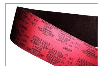
Made with finest quality of treated Aluminium Oxide grains coated on Polytex Y wt Cloth with strong and flexible bonding of synthetic resin. Available grits: 36, 60, 80, 100, 120, 150, 180, 220, 320, 400, 600. Maximum Jumbo roll width 1410mm. Backing colour red.
