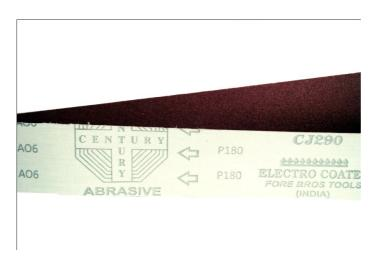
Made with soft Aluminium Oxide grains coated on highly flexible J wt Cotton Cloth with flexible bonding of synthetic resin. Grits available 60-400. Can be converted into belt, roll. Maximum Jumbo roll width 1410mm. Backing colour white.
