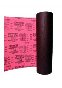
Made with Aluminium Oxide grains coated on Polytex X wt Cloth with flexible bonding of synthetic resin. Grits available 60, 80, 100, 120, 150, 180, 220, 320, 400, 600. Can be converted into Flap Wheel, Mop Wheel, Sector Wheel, Cup Wheel, Flap Disc. Not suitable for belts.
