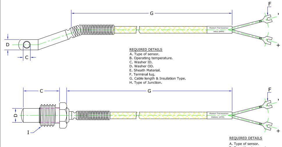
\*Suitable for extruder nozzle, motor, and pipe temp etc. these assemblies are available as all standard in thermocouple connection & calibration codes. They can be supplied Mounted into any bolt as required by an Application. Junction are normally grounded to the bolt. Exposied or Insulated can be supplied as on optional extra.
