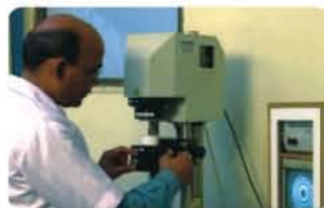
Laser Interferometer for optics inspection
