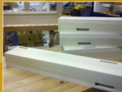
Mortising in Wood
